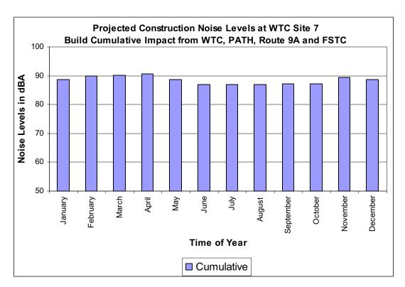
Projected Construction Noise Levels for Cumulative Effects with Proposed Action – 30 Day Leq
