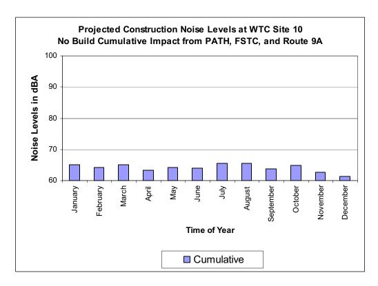
Projected Construction Noise Levels for Cumulative Effects without Proposed Action – 8 Hour Leq
