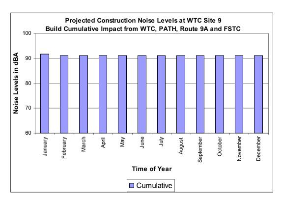
Projected Construction Noise Levels for Cumulative Effects with Proposed Action – 8 Hour Leq
