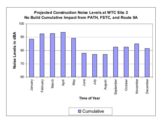
Projected Construction Noise Levels for Cumulative Effects without Proposed Action – 8 Hour Leq
