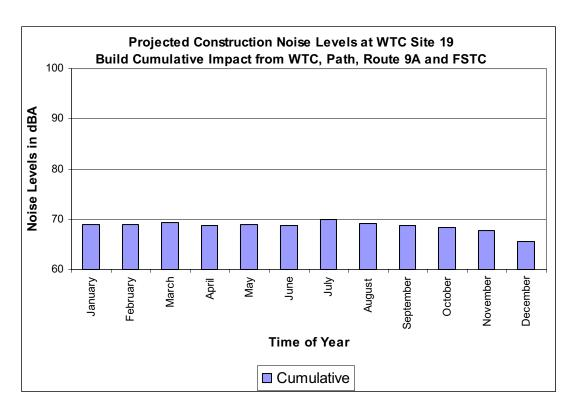
Projected Construction Noise Levels for Cumulative Effects with Proposed Action – 1 Hour Leq
