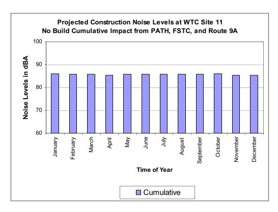
Projected Construction Noise Levels for Cumulative Effects without Proposed Action – 1 Hour Leq
